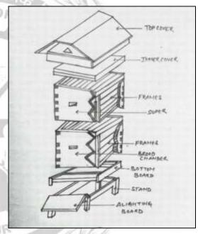
Frames: These are the wooden structure consist of a top bar, two side bar and a bottom bar, inside parts that hold the comb. The underside of the top bar is grooved to hold the comb foundation. The side bar had four holes for wiring
